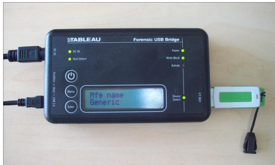
Figure 27, Tableau USB write block with USB as the source drive
